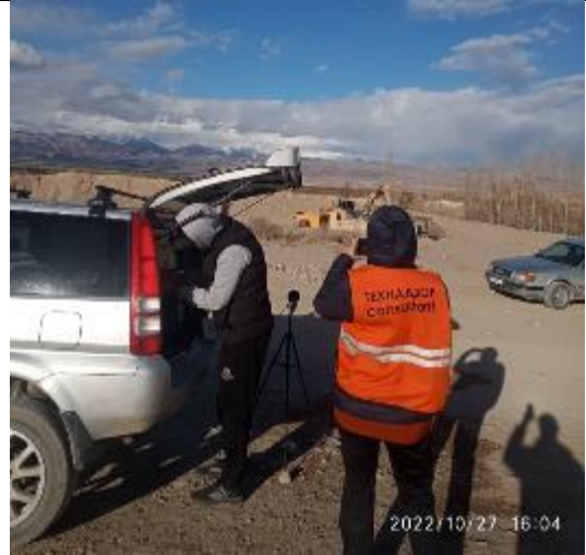
Photos 84. Lot 2. Quarry km.75+400. Noise and vibration level measurements.
