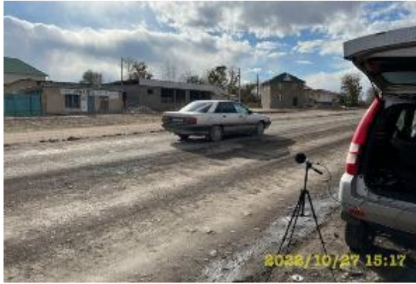
Photos 83. Lot 2. km.66+125, Kok-Zhar village. Noise and vibration level measurements.
